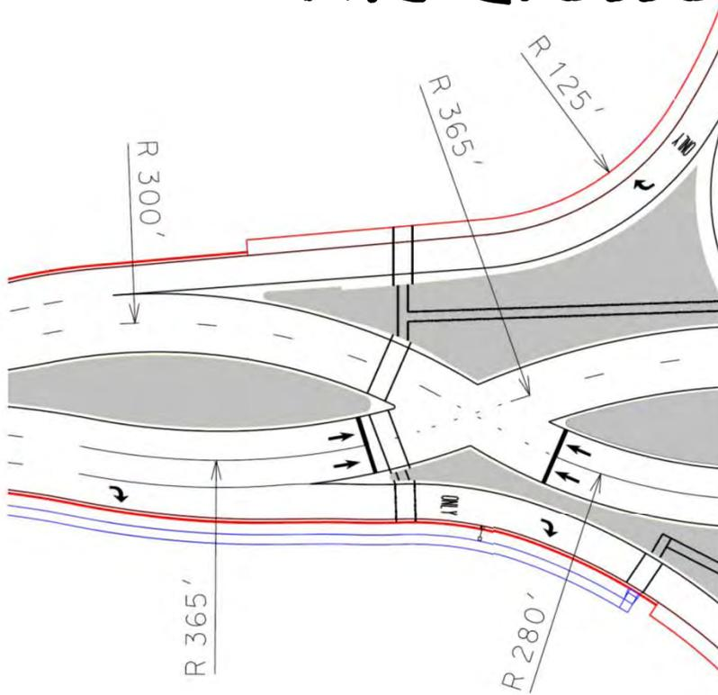
◇ Design of I-435 & Front Street DDI Crossover with larger radii to accommodate high truck/heavy vehicle %
